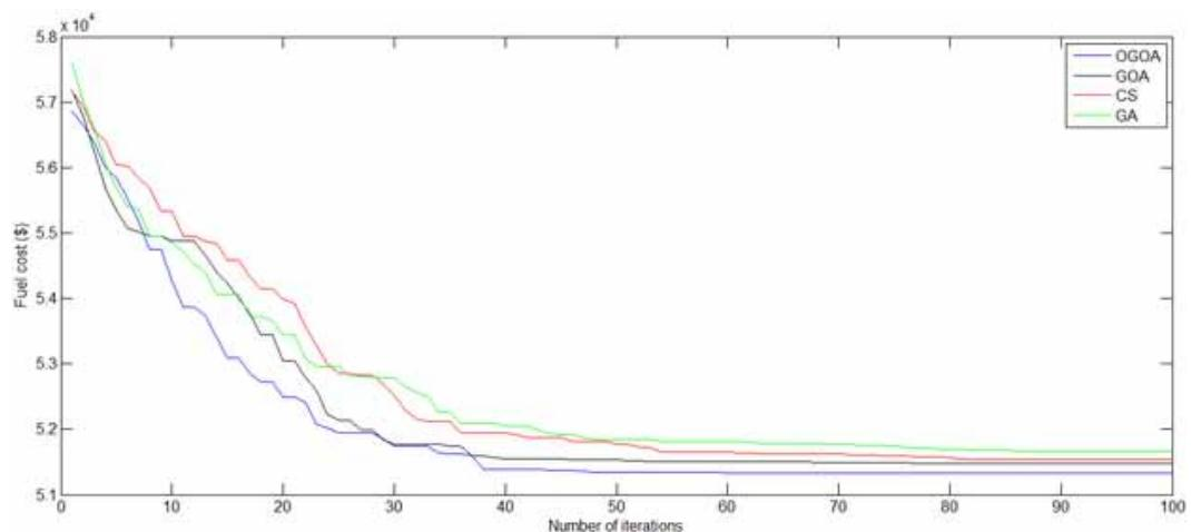
**Figure 8. Convergence graph for with wind and with emission tax of 1200 MW load using different algorithm**
